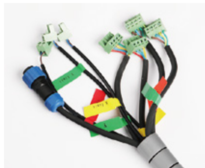
Cables to Control Box side
