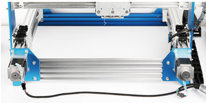
Y2 to Left Motor and Y1 to Right Motor
