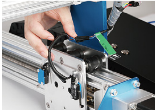
Y-Axis Limit Switches
