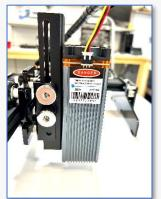
• Locate the two-piece power cord and plug it into a power source. The unit should now "home" and hit two limit switches.
