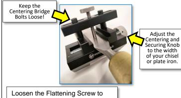
Loosen the Flattening Screw to allow for enough insertion clearance.
