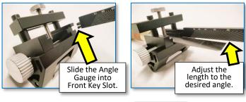
Once you are satisfied with the angle position, tighten the Flattening Screw and Centering and Securing Knob!
