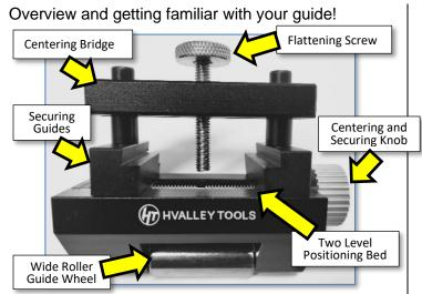
As you begin using your guide, leave the two bolts on top of the Centering Bridge sufficiently loose so that it will easily slide side-to-side.
