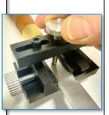
Now, you can either match the current angle of your chisel / plate iron by adjusting its length or attach the angle gauge for a more precise angle.
