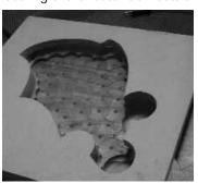
along the perimeter of the template. Turn the router off, making sure the bit comes to a complete stop before removing the router.
