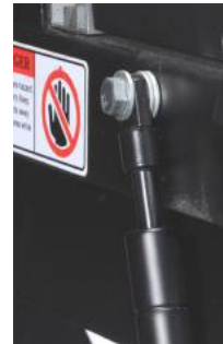
Top of Strut attached to Table
