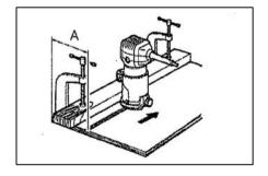
To cut a straight line, you can use a straight edge template to guide the router base. Draw a straight line on the work-piece where you wish to make the cut. Draw a second straight line parallel to the cut line back into the work-piece at the distance between the router base and
