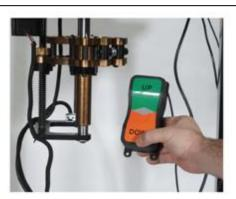
3. With the lift carriage in the lowest position insert the router motor into the carriage and lock it into place. You will want the top of the router motor just about flush with top of the carriage. Use the largest hex wrench to tighten the motor into position.
